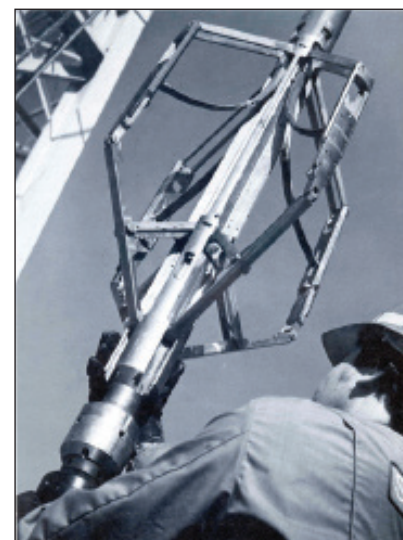
Figure 5. Four sensors, mounted on spring loaded arms that press them against the borehole wall, are pulled up the well to make the measurement. [Schlumberger]
