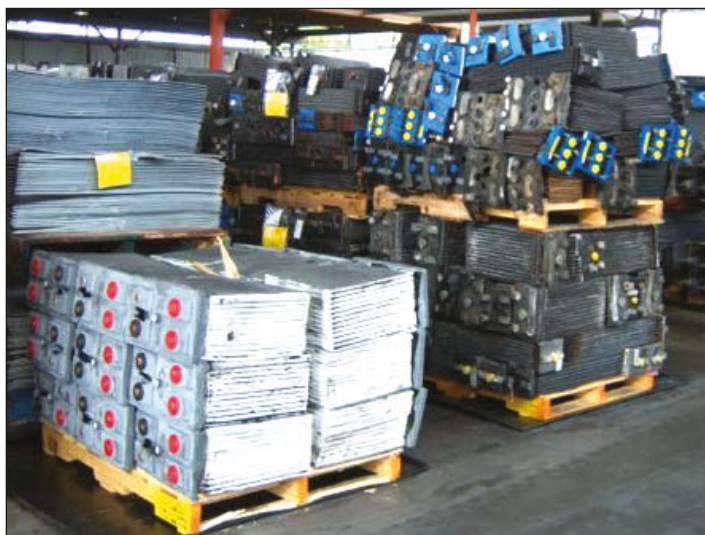
FIGURE 3: Lead-acid battery cases and plates after separation.
