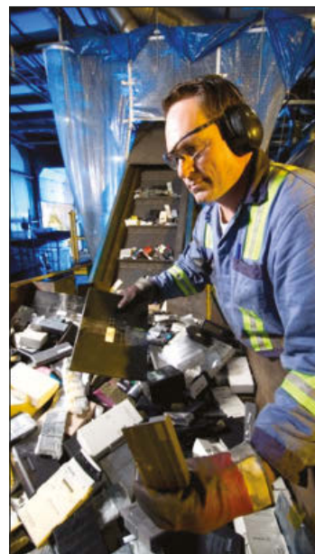
FIGURE 4: Hand-sorting of Ni-MH consumer batteries (Courtesy of Kinsbursky Brothers, Inc.)
