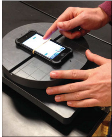
Physics lab students use the smartphone gyroscope sensor to measure angular velocity at North Carolina State University.
