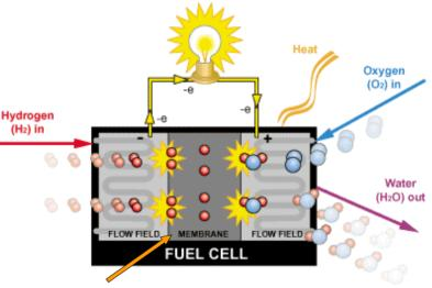
Membrane conducts protons from anode to cathode proton exchange membrane (PEM)
