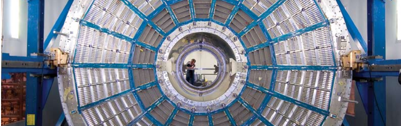
View of the ALICE Time Projection Chamber, part of the inner detector of ALICE, in a clean room. (© CERN 2005)
