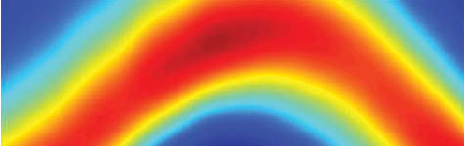
Distance vs. time plot showing atoms entering and then "reflecting" back out of an atom "mirror." (E. Vliegen/ETH-Zurich, see http://focus.aps.org/story/v18/st3 )
